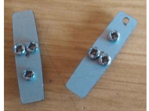
So I designed and built a jig to help keep the drill steady whilst drilling the hole. It needed to be simple and easy to use, and so this jig emerged. Soon found out that I had a mix of code 80 and 55 at various parts of the layout and found that the pitch of the sleepers was slightly different, which is why there are now 2 jigs in the set.
