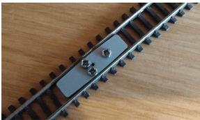
This set comprises 2 metal jigs that allow you to position track pins in the middle of the plastic sleepers on Peco n gauge flex track.
