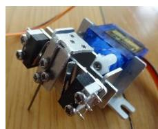
There are mounting facilities for 2 micro switches and, in another new innovation, these can be pre-assembled with the screws and nut plates before sliding them onto the
