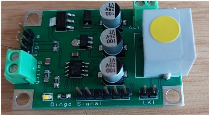
Again this is a development which is still in its early stages. I have developed a board which will do a double pull on the upstroke and bounce the signal on return.
