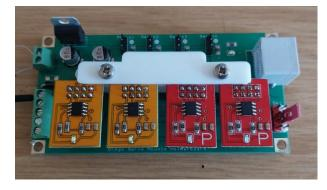
This is the first prototype which will accommodate the Power HD HD1370A servos which we use in all the mini mounts.
