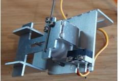
was crying out for an update. Modifications include a folded slider to operate the switch instead of the older standoff, Improved drive screw ideas as per the Mini mounts, fully slotted switch mounting to allow the switch to be assembled away from the mount and a general tidy up of tight spaces to make the mount easier to assemble.
