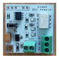
The first prototype boards have been delivered and I have built a couple to give to some friends for testing as I have never used DCC to operate accessories before. I am quite happy with the result so far and the board is quite small (33 x 33mm) and interfaces with our twin control boards as does the crossing gate sequencer.
