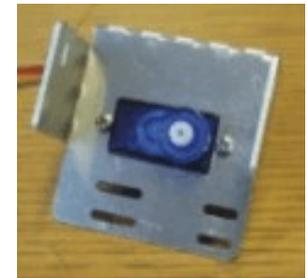
*Note: If you have folded the mount the other way (It happens) just turn the motor around to keep the drive shaft central to the switches.*
