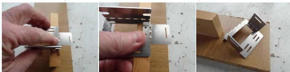
Now take the slider and fold along the short dotted line. **Take some care here as the way you fold this will determine the final arrangement of the mount.**
