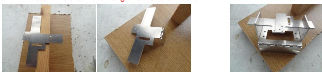
This fold is required for operating the switches if fitted. (Note: switches are not included in the kit). Now do a test fit of the two parts and make sure that the slider operates freely. There maybe a bit of a burr on the edges which can be easily removed with a small needle file.
