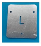
Originally I 3D printed these Jigs but now they are cut from Aluminium as per the Micro 8/10 drill jig.
