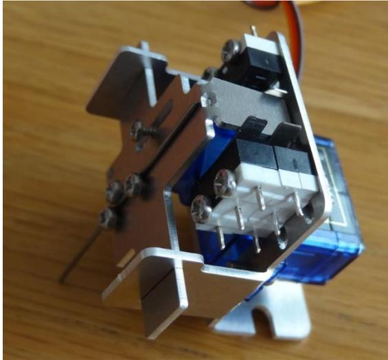
You can “double stack” the switches on the left hand side of the mount, but you will need to purchase a Long Screw Multipack with longer screws and extra switches to do this. (Screws in this pack are M2 x 16mm)
