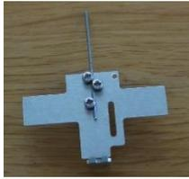
The top 4 holes in the slider are tapped M2, but we will only use 3 of them. You need to decide now which way you will use the screws to hold your actuator. (See picture) the 3 very small M2x3mm screws are used here - anything longer may interfere with the actuator arm of the servo.
