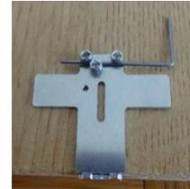
This completes the slider assembly. The actuator wire can be adjusted at any time by slacking off the screws, moving and re-tightening once in the correct position. I suggest tightening the centre screw first.
