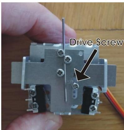
The Slider now secured to the 1.7mm self-tapping screw through the centre slot and into one of the servo horn holes. The further you go from the centre of the drive shaft - the longer the throw will be. For most points in n or OO gauge the hole closest to the drive shaft will probably suffice. This will also give you good travel on the servo motor and make setting the switches easier. There will be some play in the unit which will give a small amount of hysteresis.
