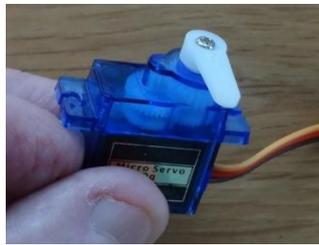
Now you need to center the servo motor. This can be done by hooking up to the servo board you are going to use to drive it or by using a servo tester unit like the small blue ones found on Ebay. These have a mode switch which will put
