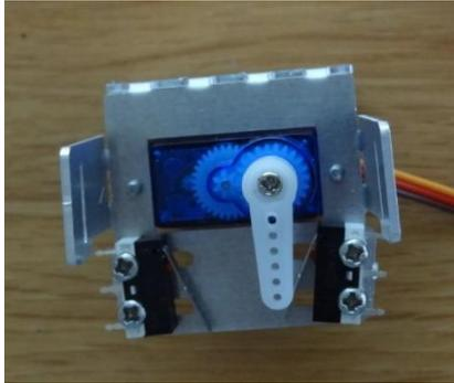
Now you can mount the motor making sure that the drive shaft is at the right hand side as shown.
