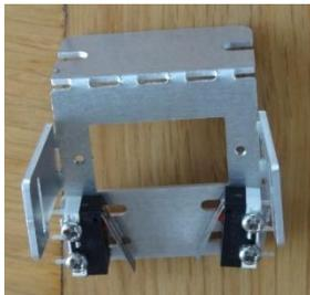
You can now fit the 2 switches to the base using 4 M2x10mm screws and the 2 nut plates. The nut plate has 2 threaded holes spaced at exactly the right pitch for the switches. This allows the switches to be adjusted very easily without having to resort to spanners etc.
