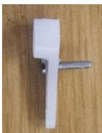
*(The object of using servos accurately in model railways, is to allow the servo a large swing, while only moving the pin a small amount. This mechanical disadvantage offers much greater control and tolerance.)*
