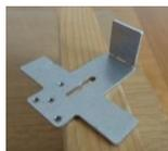
This fold is required for operating the switch if fitted.
