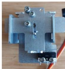
Once fitted, carefully move the slider by means of the servo tester and check that it just activates the switch as it passes the midpoint and continues smoothly over to the right.
