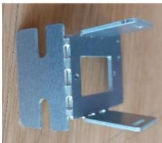
The 2 wings are bent in the opposite direction and can be bent by hand on a wooden block.
