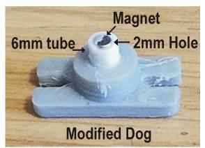
getting any glue on the outside of the tube as this need to run smoothly in the outer tube.
