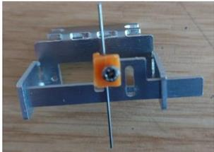
Once the slider is in place and engaging with both slots in the wings, you can gently fold the wings up to their finished position by hand. Note: if you bend them just past the 90 deg point the slider will be trapped and should move easily from side to side
