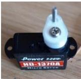
Now centre the servo with a servo tester and fit the horn as shown to the servo with the tiny screw in the servo motor pack. **(Be careful with these screws as they have a mind of their own and are hard to find replacements for)**
