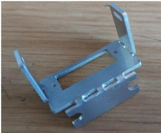
The 2 wings are bent in the opposite direction and can be bent by hand on a wooden block.
