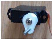
Now mount the servo motor from the back of the frame using the M1.6 x 5mm screws supplied.
