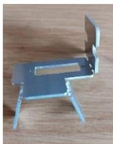
The 2 wings are bent in the opposite direction and can be bent by hand on a wooden block.
