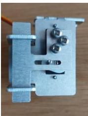
Finally fit the 3 screws on the slider for holding down the actuator wire from your signal or alternatively you may want to use the magnetic clip designed for the Omni mount as this will give more protection for your signal.
