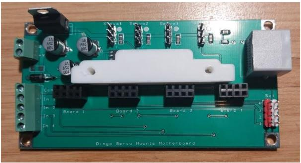
The modules plug into the board with the pins to the White plastic Clamp Make sure that the modules are plugged in correctly with all 8 pins in their respective holes.
