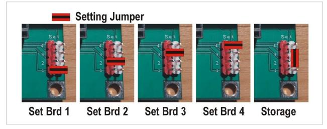
When not in use move the jumper to any 2 WHITE pins – Do NOT leave it on the RED pins.
