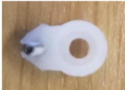
Now remove the excess length of the horn down to the second hole and trim corners with a pair of side cutters.
