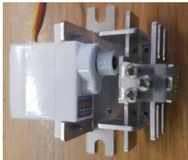
If using this as a signal driver, you will place these 3 screws as shown here. Also you will need to bend the signal side plate along the dotted line on a wooden block or on the side of the work bench to 90 deg. This is attached to the base of the mount with the remaining 2 screws (M2 x 3mm)
