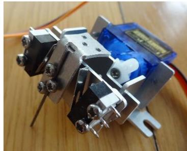
Once everything is working properly, the switches can be adjusted inwards so that they just operate at the end points of travel.
