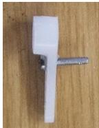
Carefully fit the 1.6mm x 8mm screw from the “servo” side of the horn through the hole closest to the boss. This should screw in quite easily but be tight once screwed all the way in.
