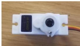
Attach with the small screw provided by the servo manufacturer. **(Be careful with these screws as they have a mind of their own and are hard to find replacements for)**
