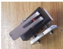
The switches can be fitted to the nut plates with the M2 x 10mm screws (Note you will need to separate the nut plates either by bending back and forth or carefully cutting with a pair of side cutters. The switches can be slid onto the mount later once it has been installed and set up.
