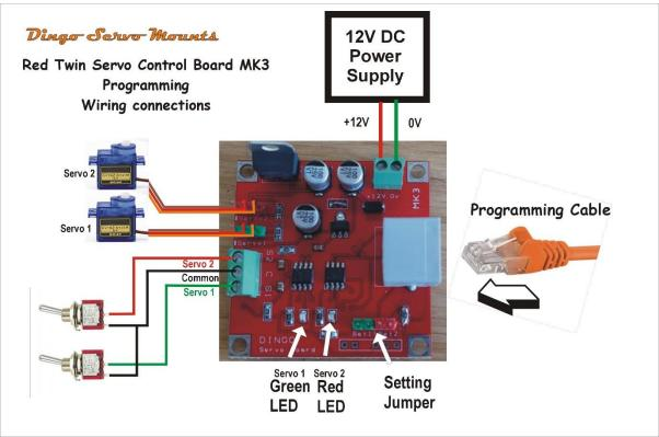
Now plug in setting box into the RJ45 connector on the board. Before connecting the setting box make sure that both controls are in the mid position. Arrows or markers pointing straight up.
