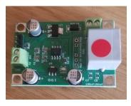
Note: A RED dot on the PCB indicates that the firmware has been updated to be compatible with the Ultra Micro Servos: HK5330 and HK282A as well as operating normal 9g servos. (HK15178, SG90, etc)
