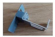
I suggest that you insert the M2 x 3mm screws for holding the actuator wires into the sliders before fitting them.
