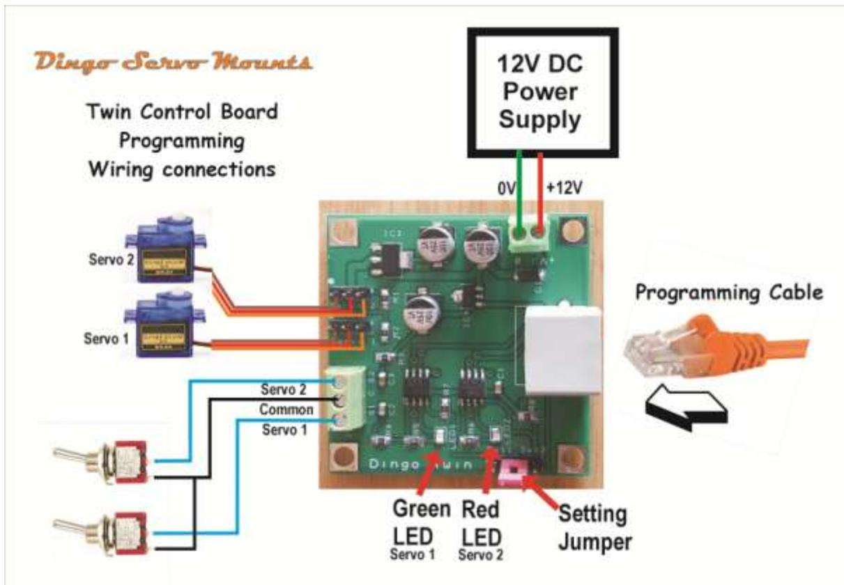
Now plug in setting box into the RJ45 connector on the board.
