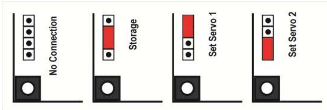
With setting Jumper moved to top position you can set Servo 1
