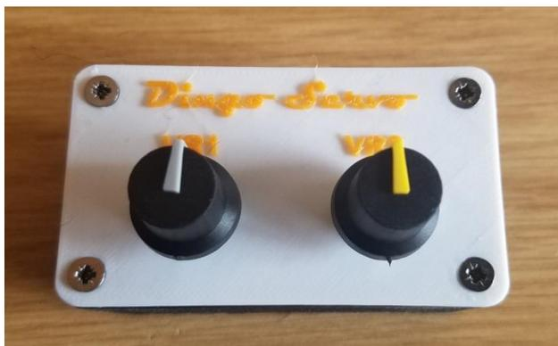
Before connecting the setting box make sure that both controls are in the mid position. Arrows or markers pointing straight up.
