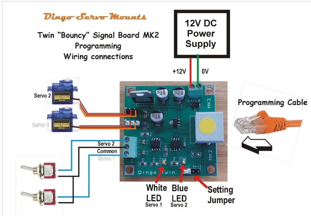
Now plug one of our setting boxes into the RJ45 connector on the board.
