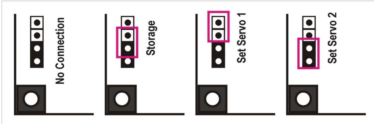
With setting Jumper moved to top position you can set Servo 1 (White Setting Pins)
