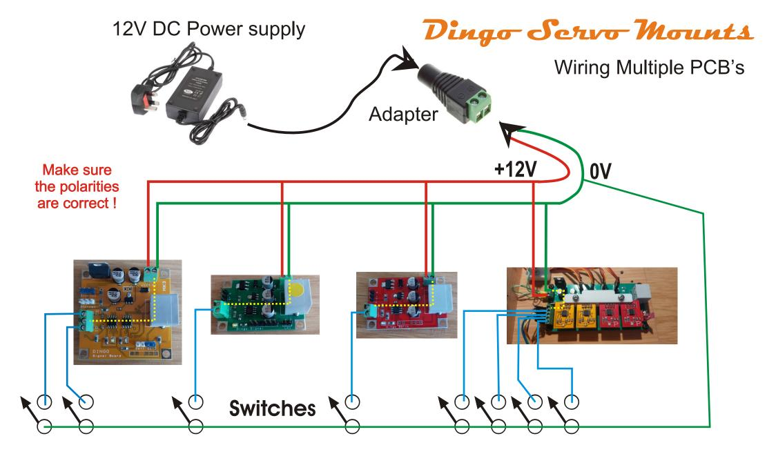
Note: It is not necessary to wire a 0V return to the boards as the "Black" marked terminals are all at 0V and are internally connected on the board (The Yellow dotted line on the diagram symbolises this internal connection and you don't have to make this externally)
