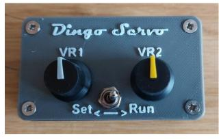
Before connecting the setting box make sure that both controls are in the mid position. Arrows or markers pointing straight up.
