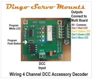
The DCC input is connected to the DCC bus on the layout.
