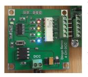
This control board came into being because I have been asked frequently to have a DCC interface to work with our standard control boards where modellers do not wish to run an analogue system for points and signals.
