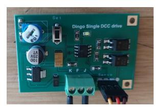
I am working with Julien Coles from France to develop a DCC operated servo control board. This board can be operated by an accessory address on DCC. It is also setup via the DCC system as well which negates the need for a setting box or similar.
