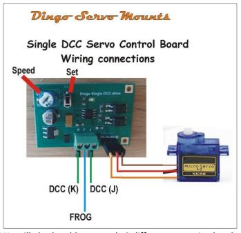
The DCC input is connected to the 2 outer terminals marked K and J
