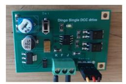
This control board is the brain child of Julian Coles, who cam up with the idea of a small single servo board controlled completely by DCC.
